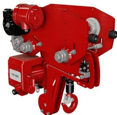
**General:** With the LHR series we have a range of trolleys for those applications where a standard trolley headroom is too large. With this special version the hoist is built into the frame of the trolley to decrease the distance of the lower hook to the beam to an absolute minimum.
