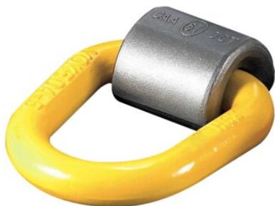
The eyes can be loaded with working load limit in all directions, pivots through 180°. Load rated parts are 100% magnaflux crack detected. Individual forged parts are traceable to Test Certification. Proof tested to 2.5 times the WLL, fatigue rated to 1.5 times the WLL. A protected spring keeps the load ring in a required position. The parts are connected in such a way that they remain captive. The spring also reduces noise caused by vibration.
