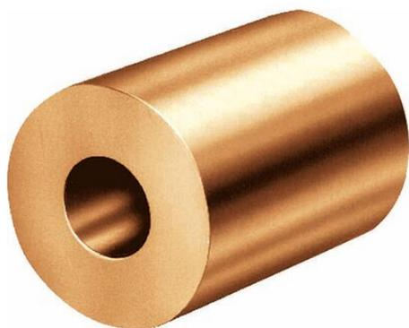
Round copper ferrule (RCU) is intended to be pressed on single round strand wire ropes, for instance on preventer wires or used as end stop. Copper as material suits well together with stainless steel wire rope, to avoid galvanic corrosion in saltwater environments.
