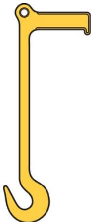
The track hook is a specialised lifting tool designed for handling and moving continuous tracks on excavators and pile drivers. Its thin profile allows easy insertion between track segments, enabling controlled lifting and positioning during maintenance and assembly work.
