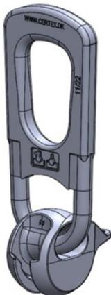
The Starcon lifting eye with universal coupling joint is used for lifting spherical anchors embedded in precast concrete elements. The spherical claw grabs the head of the spherical anchor. The lifting eye can be mounted to a crane hook or other lifting equipment. The plate can rotate around the lifting eye, which enables lifting with different inclinations. The equipment can be reused for many lifting operations.
