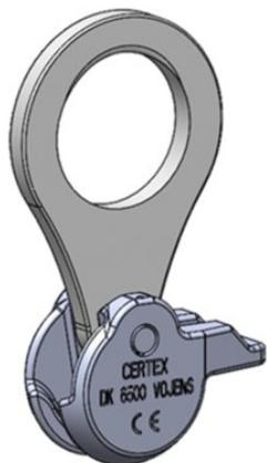
The Starcon lifting eye with standard coupling joint is used for lifting spherical anchors embedded in precast concrete elements. The spherical claw grabs the head of the spherical anchor. The lifting eye can be mounted to a crane hook or other lifting gear. The plate can rotate around the lifting eye, which enables lifting with different inclinations. The equipment can be reused for many lifting operations.
