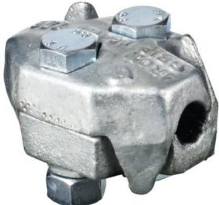
**General:** Wire rope clamp type, approved for lifting. Requires fewer clamps per fixation, e.g. two wire clamps instead of four, for 16 mm cable. Symmetrical – cannot be wrongly fitted. The clamps ensure fixation of the wire to a degree of at least 90% of the minimum breaking load of the wire in accordance with the current European standard.
