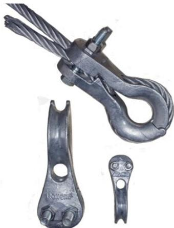
A combination of wire rope clamp and thimble, approved for application in elevators and hoists. Two part thimble and recessed bolts, for easy mounting.
