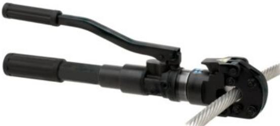
**General:** A single acting hydraulic cutting tool with a two stage built-in handpump suitable for cutting steel wire ropes. Blades are replaceable. The tool is supplied with a canvas carrying bag.
