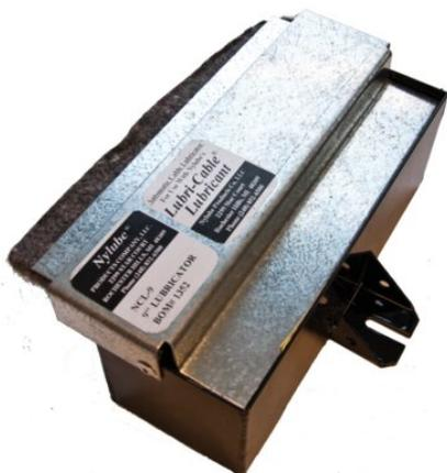
**General:** For Elevators, Escalator Chains, and Selector Tapes. Keeps cables constantly lubricated thus increases cable and sheave life. Features adjustable oiling rate-wick lock, adjustable wick length and a top fill external level indicator. Lubricates by electrostatic attraction - which means only minimum wick adjustment necessary after installation.
