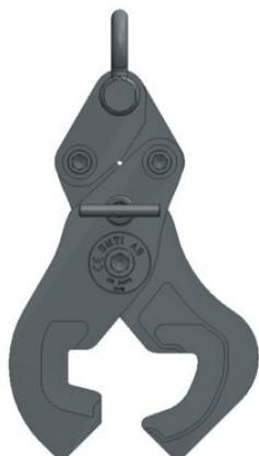
For lifting and transportation of street rails of types 57R1 and 60R2. Thanks to its clever design, which takes up minimal space, this clamp can efficiently be used for stacking a number of standing rails at a time. The clamp is locked by turning the knob placed at the flange of the rail.
