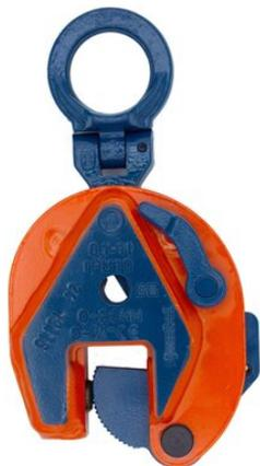
The IPU10H vertical lifting clamps are used for the lifting, turning, moving or vertical transfer of **very hard** (up to 472HV10 (450 HB) sheet, plates, or fabrications, from horizontal to vertical and down to horizontal (180°) as needed. The hinged hoisting eye ( a.k.a. universal eye ) allows for the clamp to place and lift the load from any direction, or with a multiple leg sling without side-loading the clamp. Available in a variety of models:
