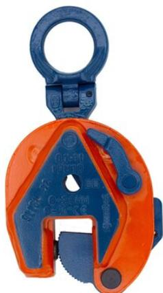
The IPU10 vertical lifting clamp is used for lifting, turning, moving or vertical transfer of sheet, plates, or fabrications from horizontal to vertical and down to horizontal (180°) as needed. The hinged hoisting eye ( a.k.a. universal eye ) allows for the clamp to place and lift the load from any direction, or with a multiple leg sling without side-loading the clamp. Available in a variety of models:
