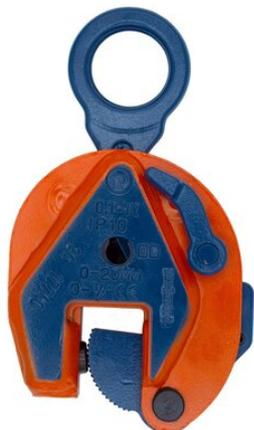
The IP10 series vertical lifting clamps are used for the lifting, turning, moving or vertical transfer of sheet, plates, or fabrications from horizontal to vertical and down to horizontal (180°) as needed. Usually used as a single point pick or when used with a spreader beam with multiple vertical drop lines. Available in a variety of models:
