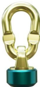
The eyes can be loaded with working load limit in all directions. All the eyes are pivoted to avoid breakage in the eyes, which also make it possible to fold it aside when it is not in use. Furthermore it has a ball beared swivel which makes the lifting eye to always stand in the correct direction to the load.
