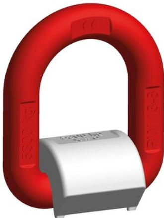
Weldable lifting point. High-tensile eyebolts pewag profilift eta, for welding onto machine parts or vehicle bodies. Ideal for hanging of lifting and lashing parts. Due to the integrated spring, the ring will be kept in each requested position.
