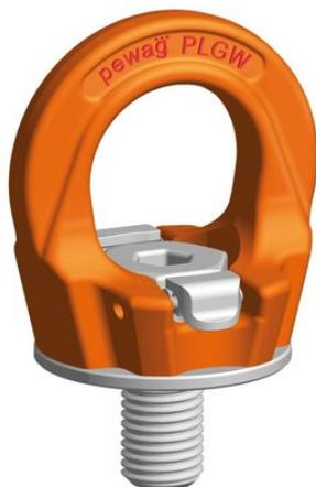
Pewag winner profilift gamma supreme – tighten by hand, then align in the load direction, a lifting point that has been developed and produced with the new standards in mind. The patented system has proven itself from the beginning. It is 360° rotatable, contains a patented and interchangeable special screw, which is 100% crack-tested as well as covered with a chrome VI-free finish-protection against corrosion and marked with WLL and thread size.
